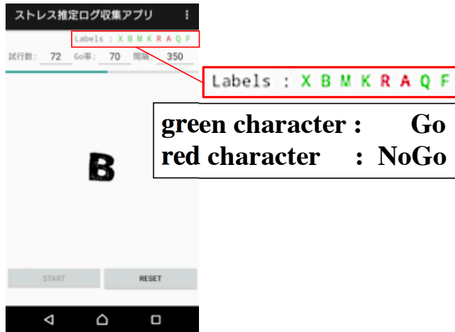
Figure 2: Go-NoGo task application; users respond by tapping the screen for “go” stimulus and suppressing taps for “nogo” stimulus.
